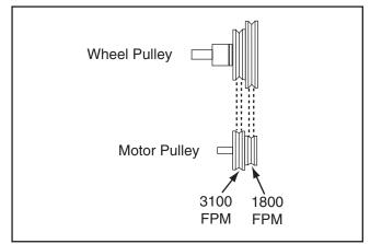
Figure 46. Belt positions for different speeds.
